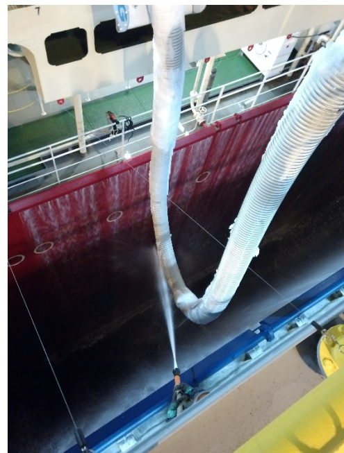
Figure 35 Hose Water spray process
