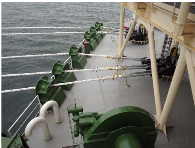
Figure 26 Stern Lines Mooring
