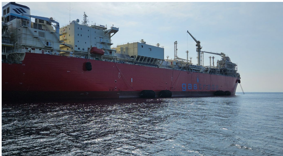
Figure 9 Primary Fender Positioning
